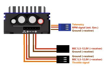
Usually in helicopters, the receiver- and BEC-cables will be wired from the front to the rear alongside the motor. Make sure that the receiver-, tele- and BEC-cables have to be wired together on one side!
