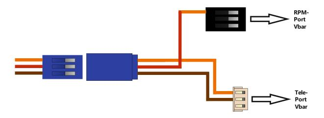
Alternatively you can use the attached long one-piece cable with all Aureus, Saphir and 205HVT speedcontrollers. For programming the ESC with the USB-adapter, please use the normal telemetry cable that comes with the ESC.
