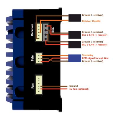
Usually in helicopters, the receiver- and BEC-cables will be wired from the front to the rear alongside the motor. Make sure that the receiver-, tele- and BEC-cables have to be wired together on one side!
